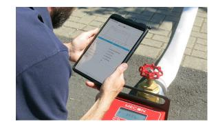
The measuring process can now be controlled not only by the easily readable display but also by the practice-proven app from wasserkarte.info. All measured data for pressure, flow, temperature and turbidity are transmitted live from the hydrant tester to the app. The measuring protocols as well as diagrams are displayed directly as preview. **The holistic solution for hydrant maintenance from documentation, planning, localization, performance to maintenance.**
